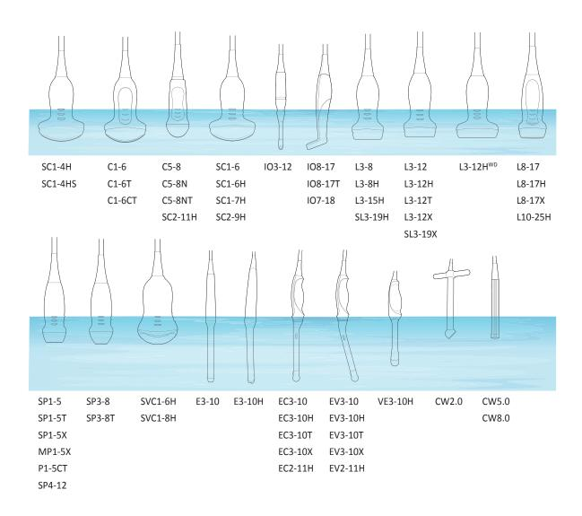
Figure 2. Transducer immersion level
