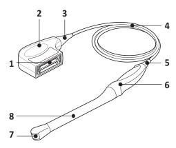
Figure 1. Transducer components
